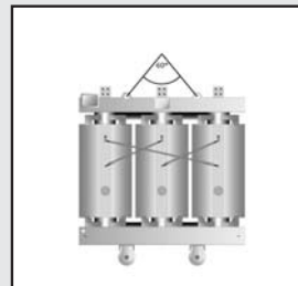
Fig. 9 Handling by means of any overhead-travelling crane
